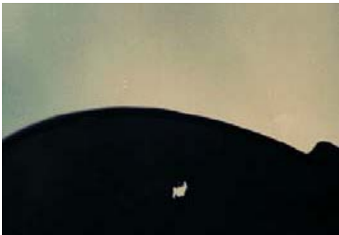
19 mm crater in the High-Gain Antenna of the Hubble Space Telescope
